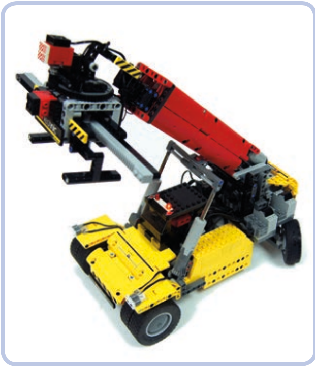
Figure 1-5: My reach stacker model had a rear axle (right) with a particularly large steering lock, just like that of a real vehicle. Designed to stack containers in ports' loading areas, reach stackers need to be able to maneuver in limited space.
