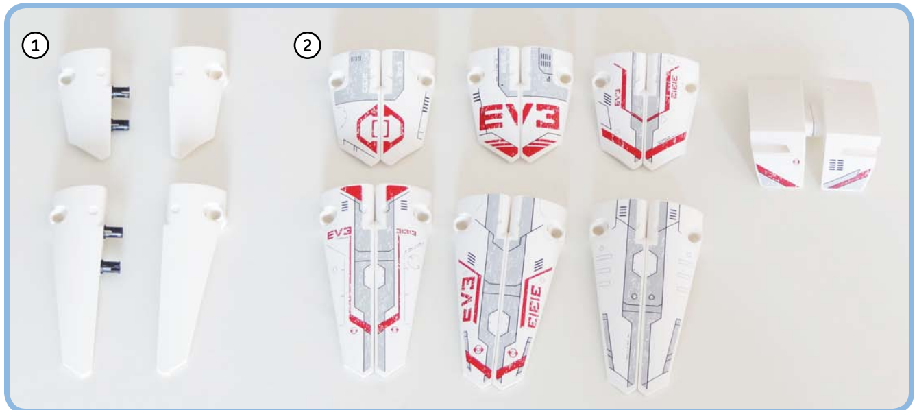
Figure 1-5: To add the stickers to the panels neatly, first connect complementary panel elements using two black pins, making it easier to align the stickers, and then remove the pins when you're done.
