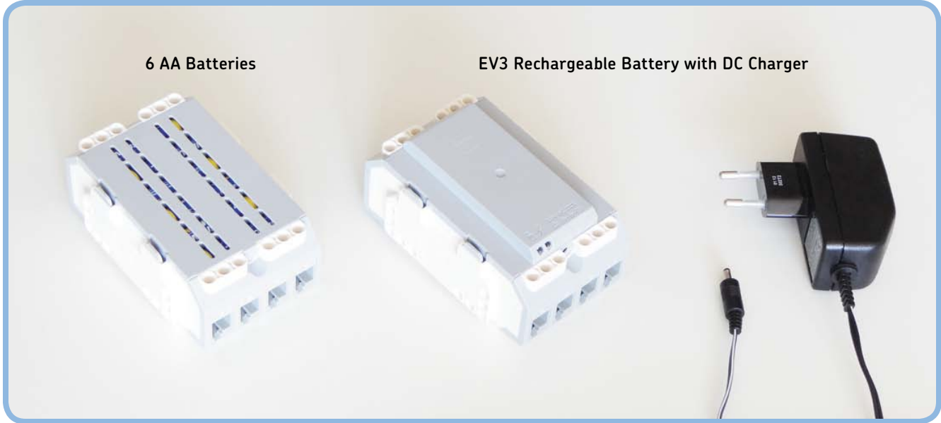
Figure 1-3: You can power the EV3 brick with six AA batteries or with the EV3 rechargeable battery.
