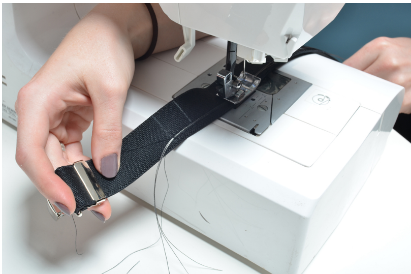
Figure 1-7. Use a sewing machine to zigzag over conductive threads
