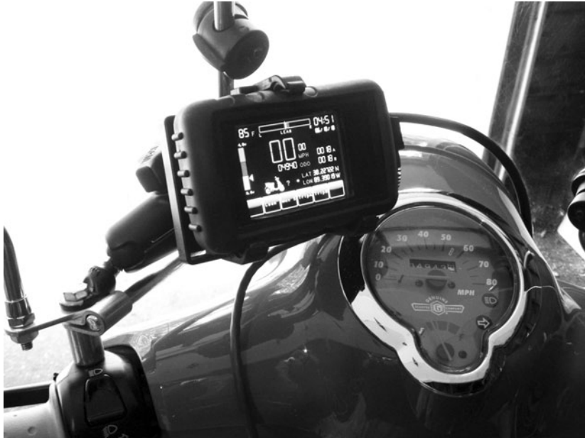
Figure 1-4: The Scooterputer display (courtesy of Kurt Schulz)
